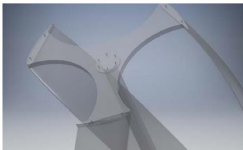
Figure 17. Attachment points of the APP parts. Source: The authors (2021).
